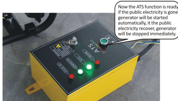
Now the ATS function is ready, if the public electricity is gone, generator will be started automatically, if the public electricity recover, generator will be stopped immediately.
