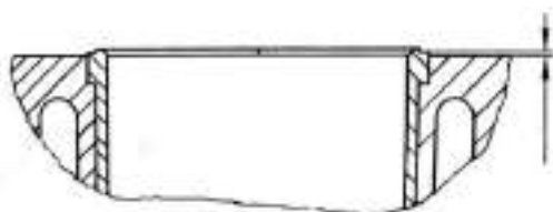
Fig.6 protruding height of the liner flange plane relative to the plane of cylinder block
